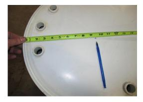
MEASURE / MARK CENTER OF CHLORINATOR BOTTOM.
