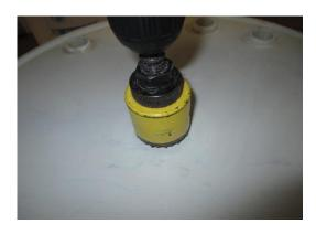
DRILL HOLE WITH 2" HOLE SAW.
