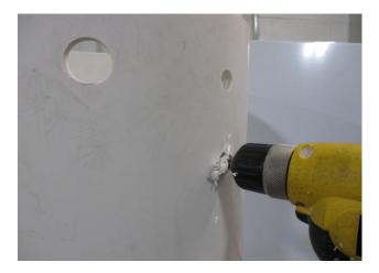
2. Tap holes with ½" NPT tap. Be careful to drill and tap the holes straight. Remove any debris from the tank when finished.
