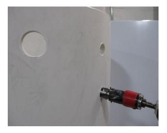
3. Using Teflon tape, tape and install the two level switches in the tapped holes. The top switch hangs down or open, and the lower switch hangs straight or closed.
