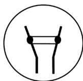
IEC 60947-5-1 Mechanically linked contacts
